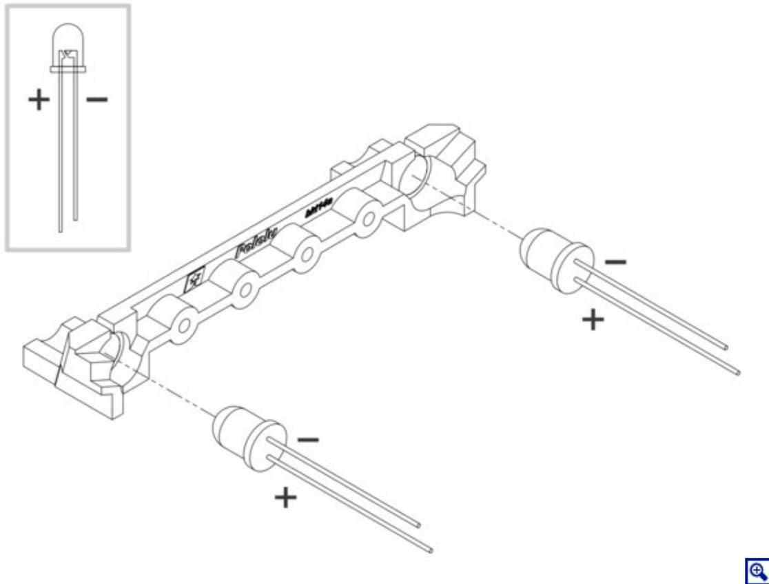
30. Bend the LED leads outward so they rest along the channels in the LED holder, then downward around the sides of the holder. Using a pair of long-nose pliers can help you make more precise bends.
