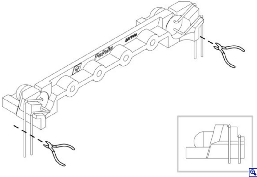
32. Install the LED holder behind the blade by inserting the LED leads into the machine pin sockets in the front of the main board.
