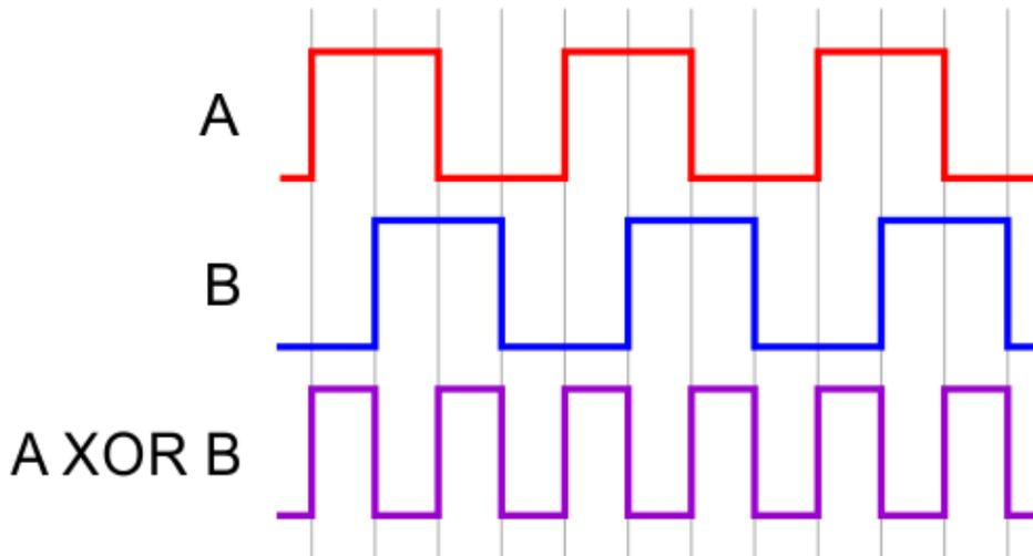
The XORed signal and the channel B signal can be used to reconstruct the channel A signal by simply XORing them again:  $(A \text{ XOR } B) \text{ XOR } B = A$ . For both encoders, channel A leads channel B when the motor is rotating in the forward direction; that is, A rises before B rises and A falls before B falls. (The waveforms in the diagram above would be produced by forward rotation.)
