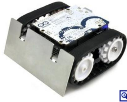
**Assembled Zumo robot for Arduino with an Arduino Uno (with original white sprockets).**
