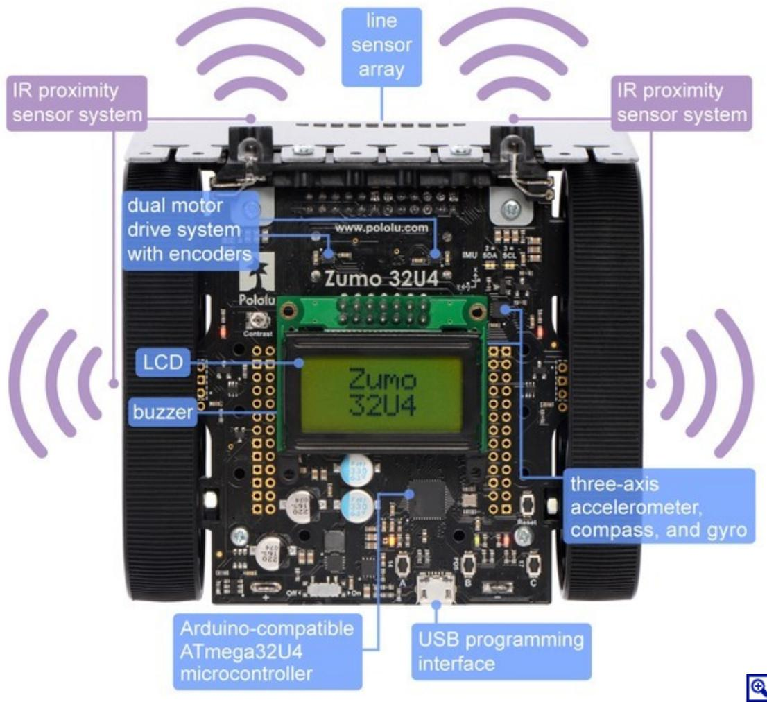
The Zumo 32U4 robot is a complete, versatile robot controlled by an Arduino-compatible ATmega32U4 microcontroller. When assembled, the low-profile tracked robot measures less than 10 cm on each side, making it suitable for Mini-Sumo competitions.
