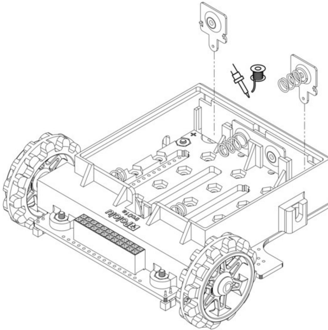
14. Solder the two individual contacts to the main board from the top. Note that if you are using a battery to hold the contact in place during soldering, the battery might act as a heat sink, making it more difficult to solder or requiring a higher soldering iron temperature. The battery terminal slot in the PCB should be completely filled with solder.
