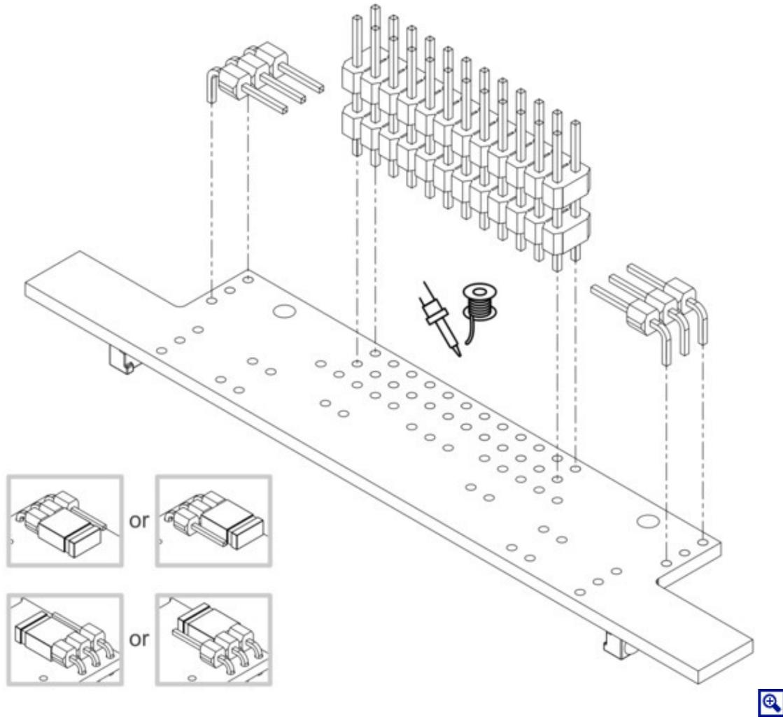
26. On each 1×3 header, install a shorting block to connect the sensor of your choice. (See **Section 3.5** for details.)
