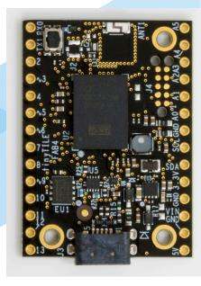
tinyTILE is a miniaturised adaptation of the Arduino/Genuino 101 board, measuring approx 35 x 26mm.
