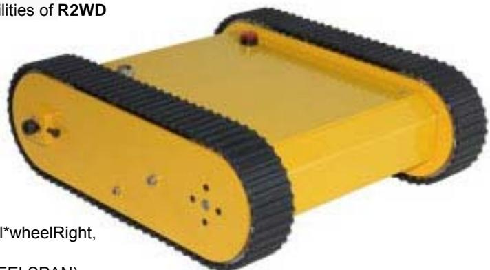
**RB015\_Tracked Mobile Tank Robot Kit**
