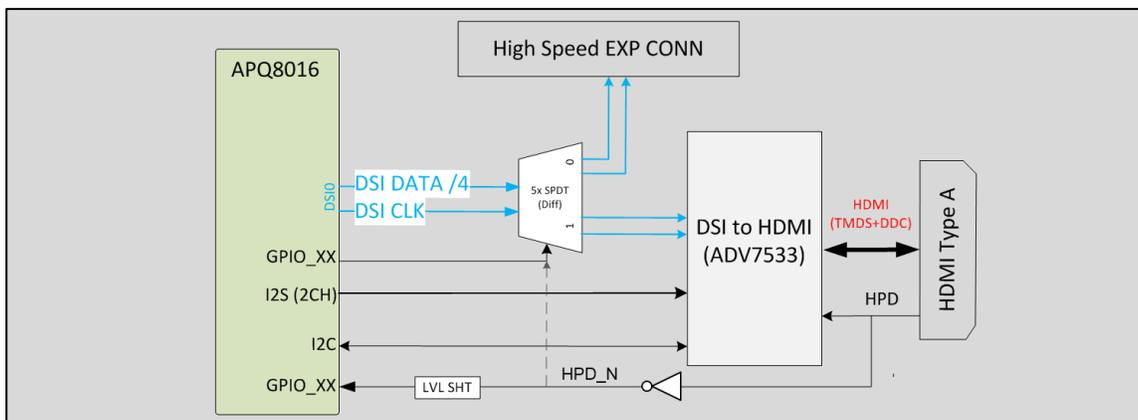
The 96Boards specification calls for a MIPI-DSI to be present on the High Speed Expansion Connector. A minimum of one lane is required and up to four lanes can be accommodated on the connector.
