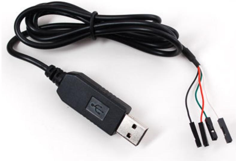
For this experiment, the serial lead is going to power the Raspberry Pi. So, **DO NOT** attach the Pi's USB power adapter. If you would rather power the Pi from your USB power adapter then leave the Red lead from the Serial lead un attached.
