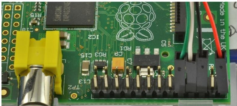
The connections are to the outside pin connections of the GPIO header. See Lesson 4, for more information about the header: <http://learn.adafruit.com/adafruits-raspberry-pi-lesson-4-gpio->
