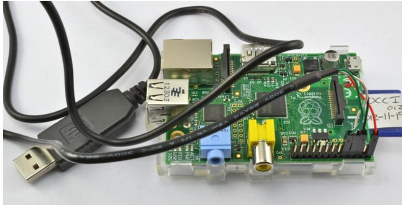
The great advantage of connecting this way is that it can even supply the power for your Pi and you do not need keyboard, mouse or display attached to the Pi to log into it.
