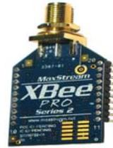
The modules operate within the ISM 2.4 GHz frequency band and are compatible with the following:
